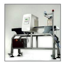
**MDF** Metal Detector is designed with a system formed by a conveyor belt or, in alternative, only the metal detector head may be supplied to be installed on existing conveyor belts or on external devices.
