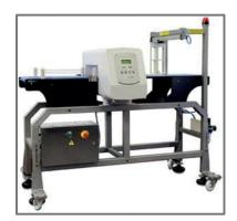
**MDF** Metal Detector is designed with a system formed by a conveyor belt or, in alternative, only the metal detector head may be supplied to be installed on existing conveyor belts or on external devices.
